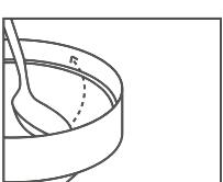
The slight edge on the inside of the bowl acts as an indicator for users with visual impairment. When scooping along the inner wall, the edge signifies to the user to stop.
