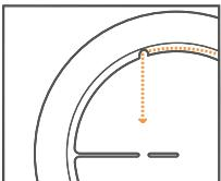
The sensory guide is a small indent on the rim of the plate that allows users with vision impairment to easily locate the partition.
