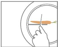
By sliding the utensil between the gap of the partition, users can easily cut through their food using one hand.
